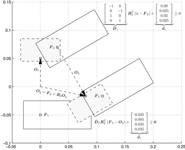
Fig. 1. Constraints on the ZMP and position of the feet.  $F_i \in \mathbb{R}^2$  and  $R_i \in \mathbb{R}^{2 \times 2}$  define the position (of a point of interest) and orientation of foot  $i$  relative to the world frame.  $O_L$  is an offset defining the position of (a point of interest of) the constraint for foot  $i + 1$  relative to foot  $i$  (expressed in the local frame fixed in foot  $i$ ).
