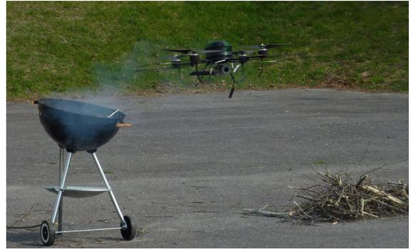
Fig. 1. Pollution source and micro-drone during one of the experiments.
